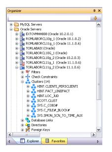
From a purely visual perspective, you can color-code individual datasources according to customizable schemes, for example to easily discriminate among, production, testing, and development servers. The explorer display can be filtered by object name or type, helpful for ad hoc visual searches or for sites with large numbers of datasources.
