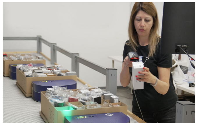
Highlighting the goods on the carrier with pick-by-light
